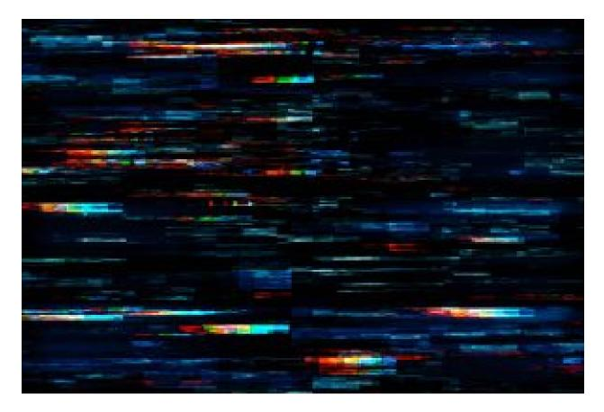
The good news is that there are just two typical root causes — interference from ambient lighting or electrical interference. The bad news is that the latter can be tricky to diagnose.
