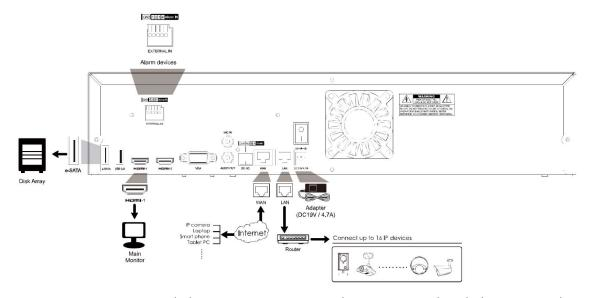
Type 2: PoE ports are provided to connect IP cameras. Then, power on the whole system and wait till the system initialization is done.
