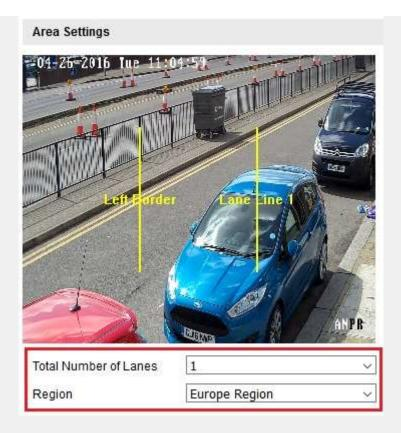
The area between these two yellow lines is the detection area the camera will monitor. It's not absolute - the camera will pick up plates from a small area outside of the detection area.
