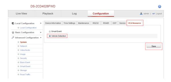
3. Then login to NVR and go to *Vehicle Detection* option. Select the detection type from the list.
