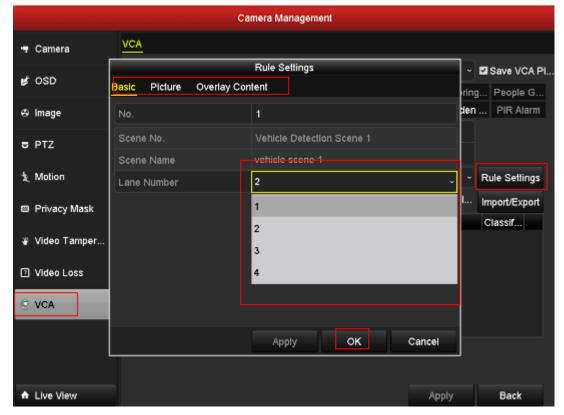
Go to VCA->Picture and VCA->Overlay Content, configure the parameter as follows.
