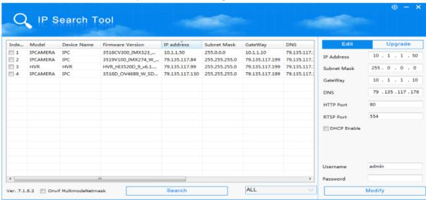
3) Now select a camera, untick the "DHCP Enable" button so you can manually change the IP.
